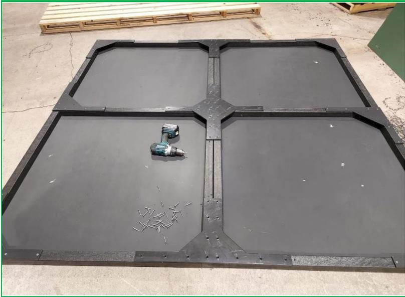
1a. There are 3 brackets to screw both floors together. Now flip the floors over and you are ready to build.
