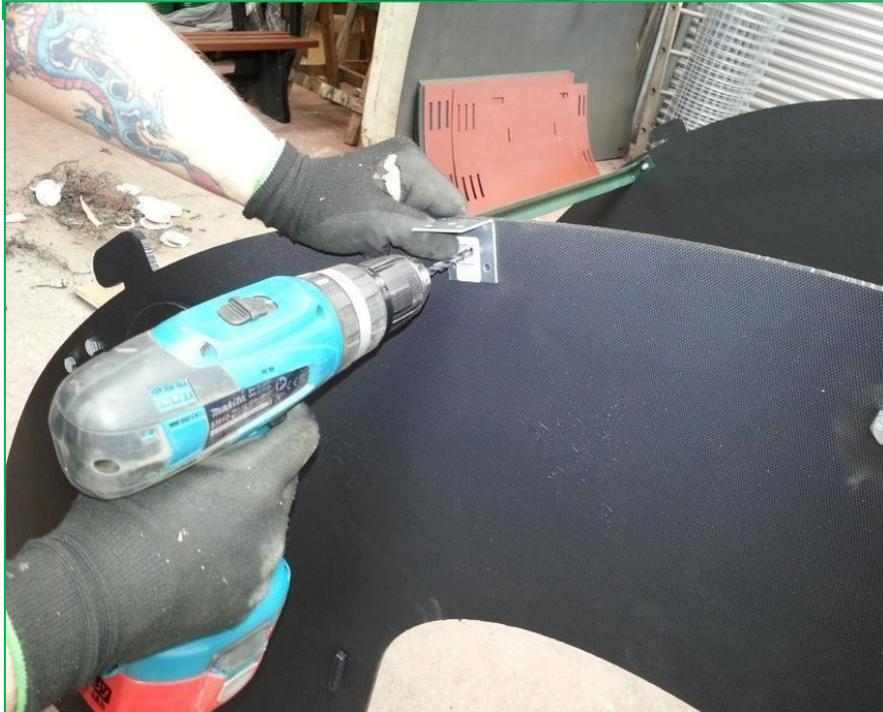
8. Pre drill holes for the metal angles to hold the roof tight against the front and back. The central hole on each side of the metal angle is one which is to be used. Use the 25mm bolts and square nuts to hold these in place. Use the bolts on the outside for a better finish.
