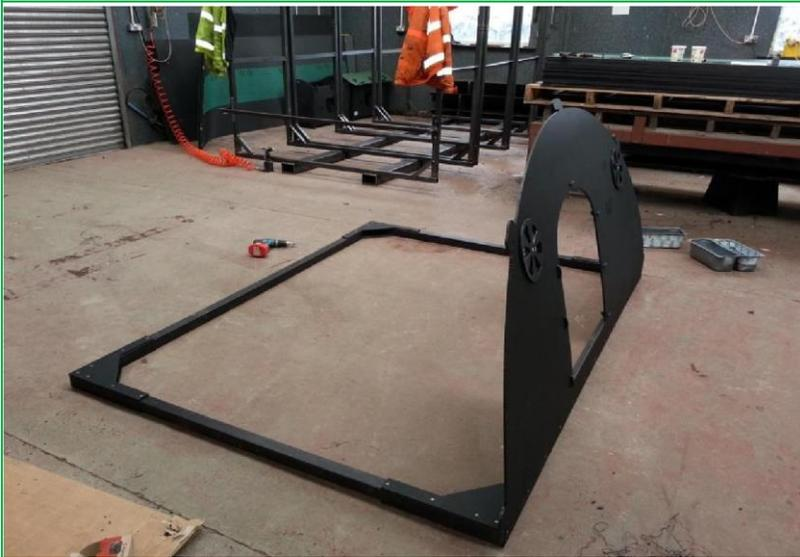
2. Attach front to floor using screws along the bottom. Ensure base of front is flush with the bottom and sides of the floor.
