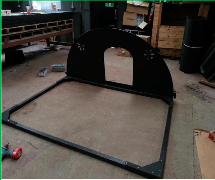
3. Attach front to floor using screws along the bottom. Ensure base of front is flush with the bottom and sides of the floor.
