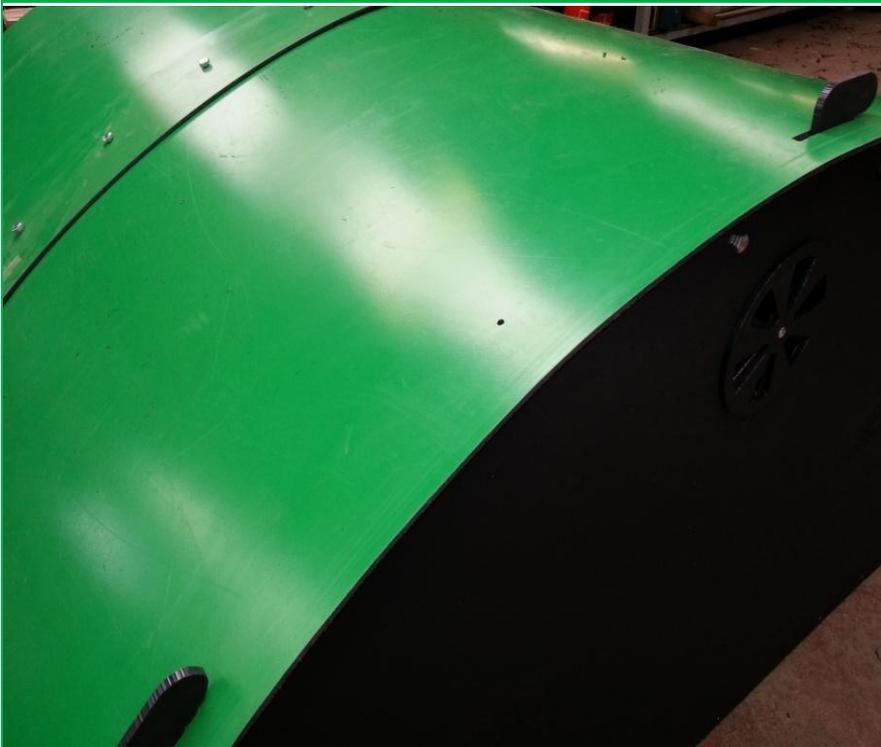
22. Drill through the central hole again through the roof panel. Use 25mm bolts and nuts to secure metal angles in place. Again, use the bolts on the outside for a better finish.
