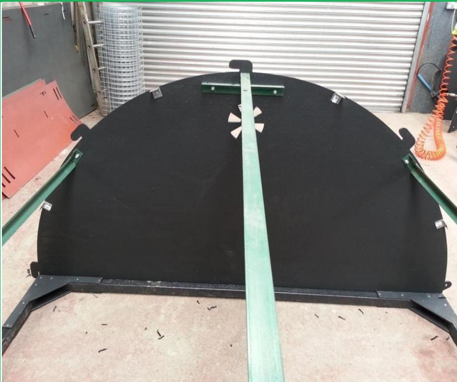
9. The metal angles go on the inside of the front and back; 4 on the front and 4 on the back. See image opposite as to where the angles should be attached. This applies to both front and back.
