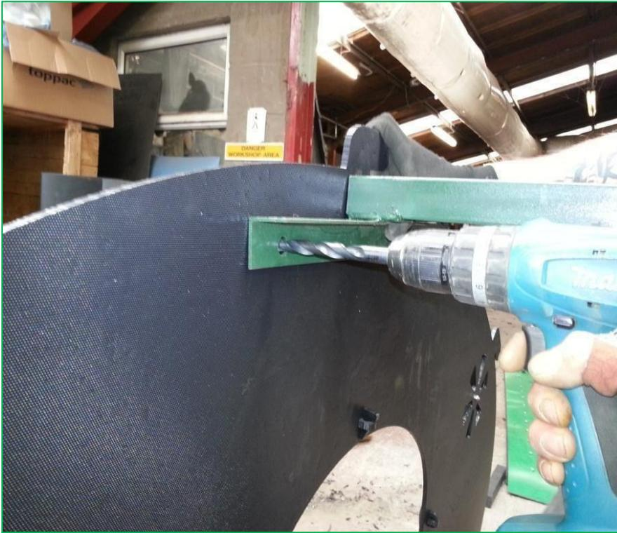
5. Line up top metal support bar so that the centre of the bar is in line with the top lug on both front and back. Holes should be pre drilled to allow a bolt to come through from the outside. Tighten nut on the inside.
