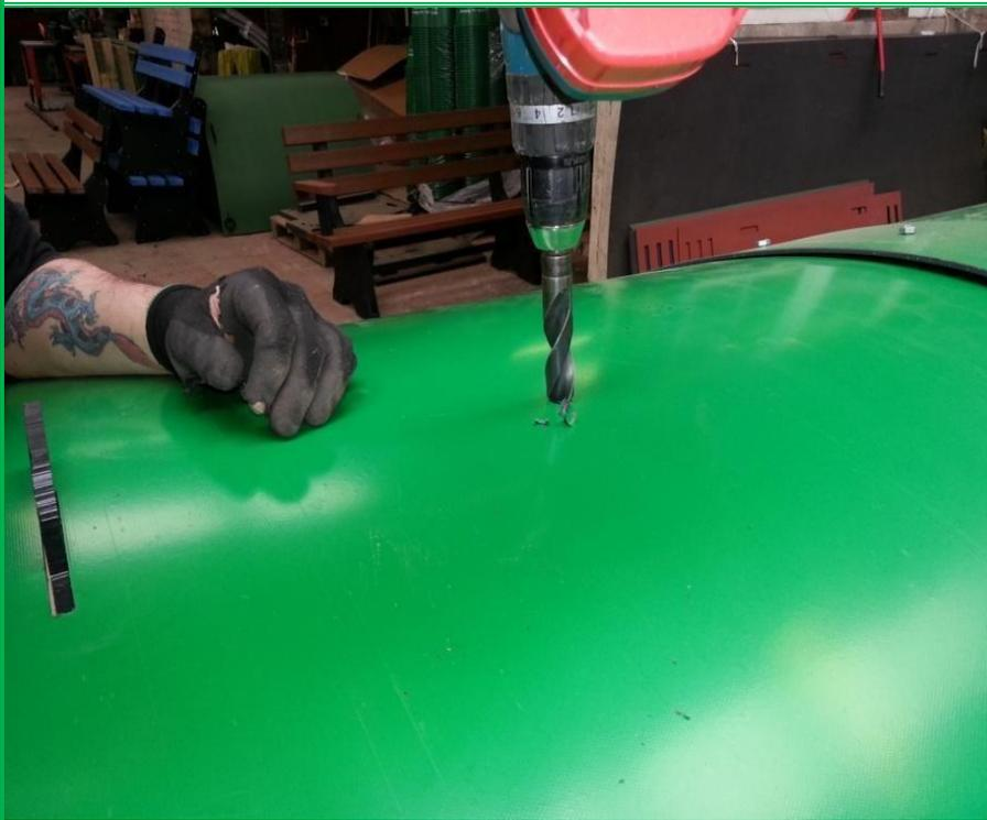
24. Drilling with the larger drill bit can be done from the inside or out as long as the original hole is central to the hole in the bar.
