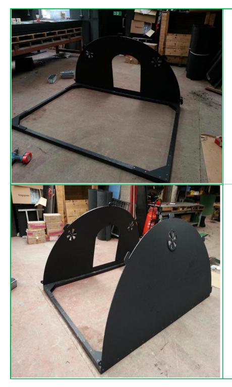
3. Attach front to floor using screws along the bottom. Ensure base of front is flush with the bottom and sides of the floor.
