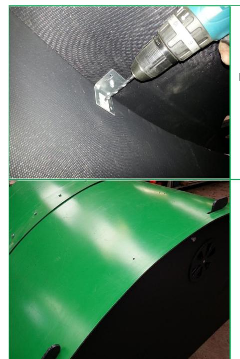
21. For the next part you have to physically climb inside the pig ark. The metal angles previously attached to the inside of the front and back are to be connected to the roof panels.
