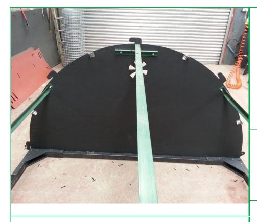
9. The metal angles go on the inside of the front and back; 4 on the front and 4 on the back. See image opposite as to where the angles should be attached. This applies to both front and back.
