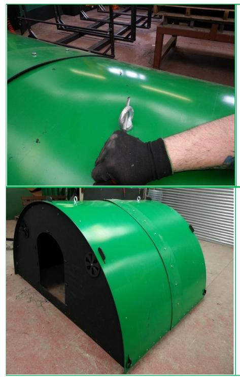
25. Slot the lifting eyes through the hole in the roof and the hole in the metal bar. Tighten the bolt from inside the pig ark while someone is holding the lifting eye straight from the outside.
