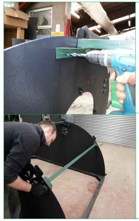
5. Line up top metal support bar so that the centre of the bar is in line with the top lug on both front and back. Holes should be pre drilled to allow a bolt to come through from the outside. Tighten nut on the inside.
